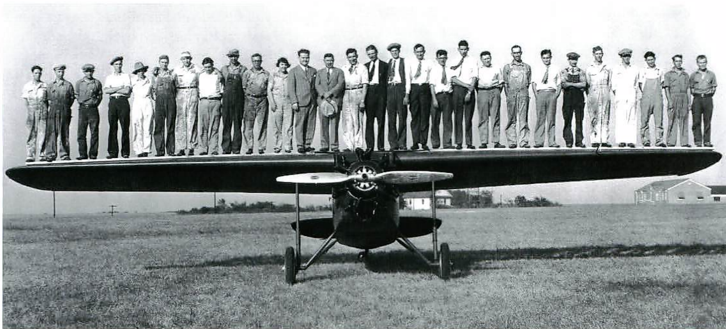
TAKEN IN 1927, THIS FAMOUS PHOTO ADVERTISED THE STRENGTH OF HIS INNOVATIVE FULL-CANTILEVER WINGS (NO WING STRUTS), CLYDE CESSNA HAD 26 MEN AND 2 WOMEN STAND ON A PLANE’S WING IN A PUBLICITY STUNT TO SHOW THE STRENGTH OF WHAT WAS THEN AN UNUSUAL NEW AIRPLANE DESIGN.
