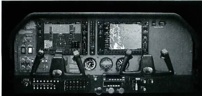
ALL CURRENT PRODUCTION CESSNA SINGLE ENGINE PISTON AIRCRAFT ARE AVAILABLE WITH THE FULLY INTEGRATED, ALL-GLASS GARMIN G1000 AVIONICS SUITE.
